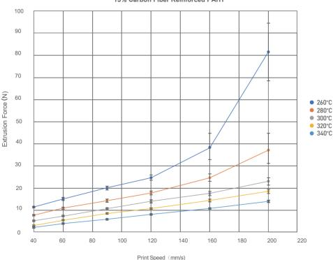
Test parameters: 12mm length brass heat block, BMG extruder, Hardened Steel Nozzle, Nozzle size 0.4mm, Layer Height 0.2mm.
